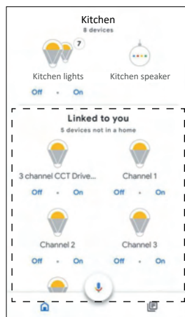
15. Adding Additional Smart Drivers If you add any additional Smart Drivers to the Link Sensio App, they will appear automatically on the Home page under the heading 'Linked to you'. You can add the new devices to a room by pressing on them and selecting a room. Alternatively, you add the devices to a room by following stage 14.
