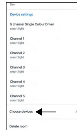
14.3 Choosing Devices From the Room Setting page, you can also select any new devices you want to assign to the room by pressing 'Choose devices'.
