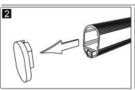
If the unit needs cutting. Remove and cap from left side only. IMPORTANT ensure sensor and on/off switch are to the right hand side facing out. DO NOT CUT FROM RIGHT HAND SIDE OF LIGHT UNIT. This will damage the internal wiring
