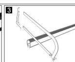
Saw light unit to correct length allowing for endcap and bracket length.
