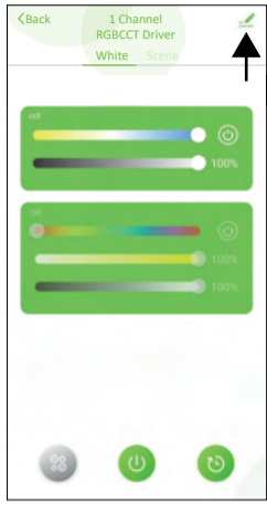
6. Connecting to Alexa and Google Assist From the Smart Driver Control Menu, press the pencil icon at the top right of the page.
