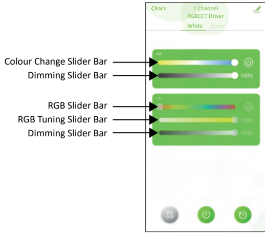
The diagram above explains how the control slider bars work for each function. Please note: The RGB tuning slider bar mixes the RGB colour with different shades of white.
