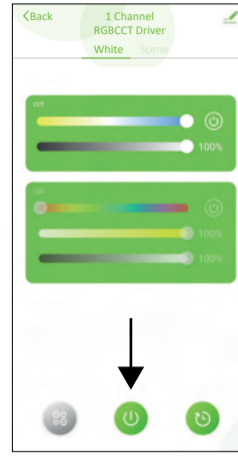
The Driver can be turned on/off by pressing the power button located at the bottom centre of the page
